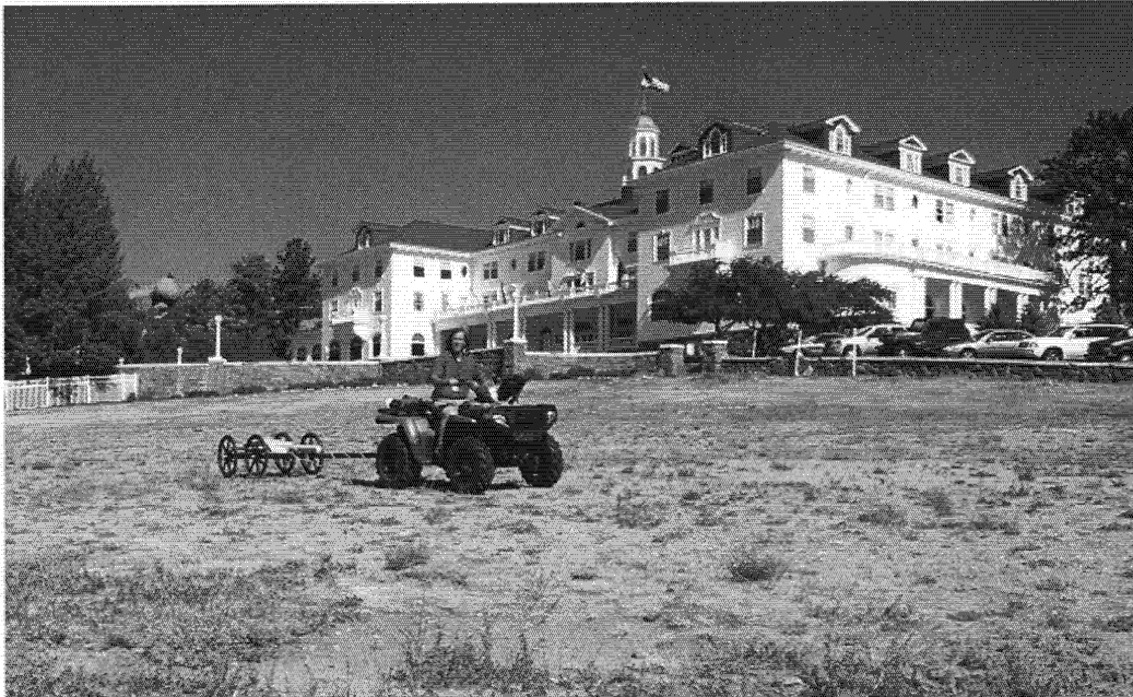
Photo 2. Jason Peel, Irrigation Water Management Specialist, (USDA-NRCS) completes a mobile EMI survey with the Dualem-2 meter at the Stanley Hotel, Estes Park, CO. The EMI mobile acquisition system observed in the photo consists of an ATV, an EMI cart, a Dualem-2 meter, a Garmin Map 76 GPS receiver, and a Hewlett Packard tablet PC. Mobile conductivity surveys are much more efficient than pedestrian surveys in survey areas containing large acreage.
